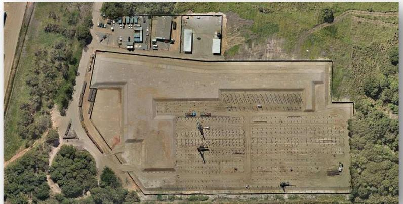
**Description:** Rolls Royce factory lies in the Sepetiba Bay area and was built on 15 m deep soft clay overlying dense sands. Therefore, Terratek designed a ground improvement solution with 1.5 m spaced wick drains and a 1.5 m temporary surcharge. All buildings were piled with nearly 30 m long steel H piles.
